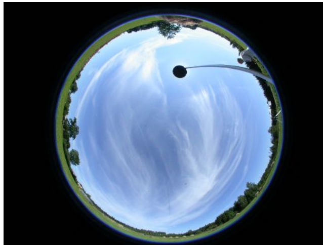
Figure 2. An hemispherical image taken with leveled camera from tripod. The field of view extends below horizon. The direct radiation from the Sun is screened to avoid artifacts due to significant scattering in the optical system.
